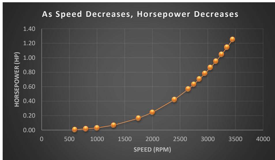
Figure 1: As the speed of the motor decreases, the horsepower required to run the pump decreases
